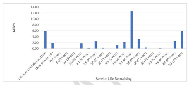
Chart 10-4: Recycled/Non-potable Water Pipeline Remaining Service Life
