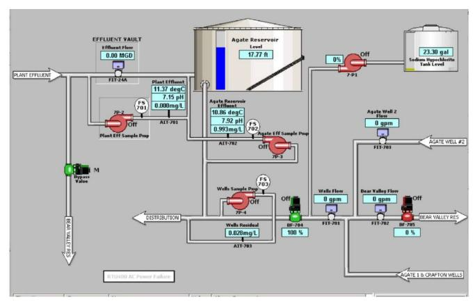
Figure 13 Agate Reservoir SCADA Layout
