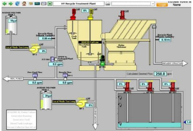
Figure 1 The Wash Water Recycled Water Treatment Plant
