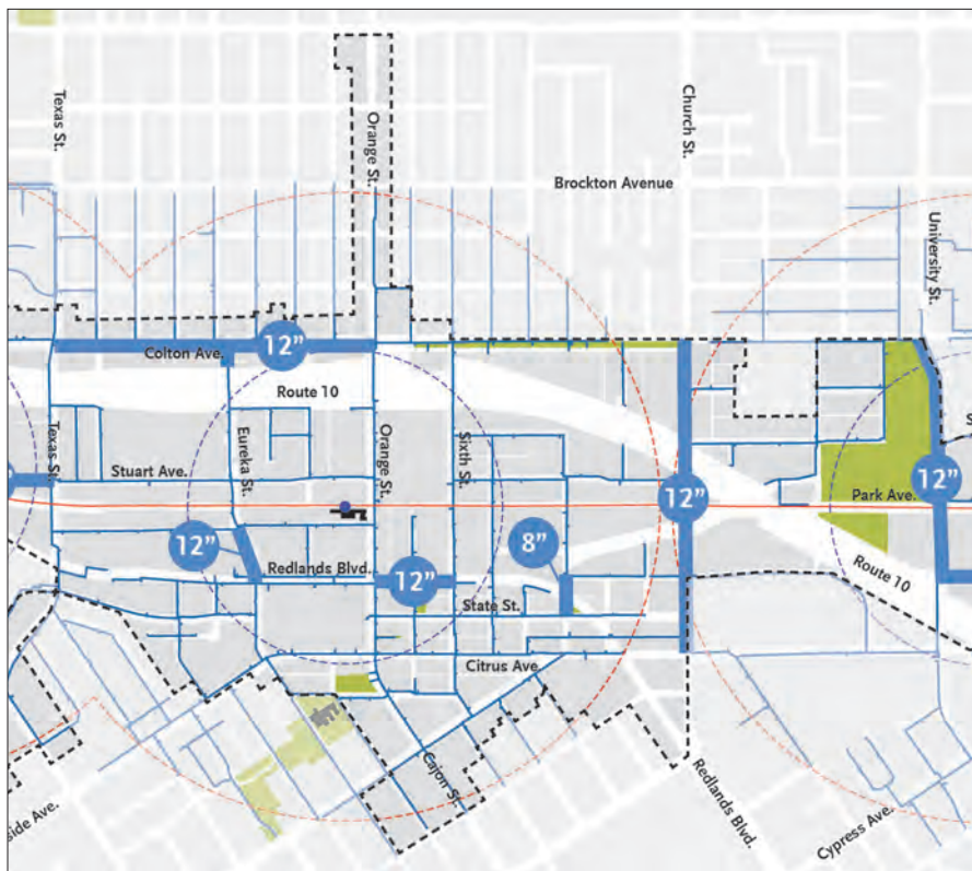
Detail of potable water network.
