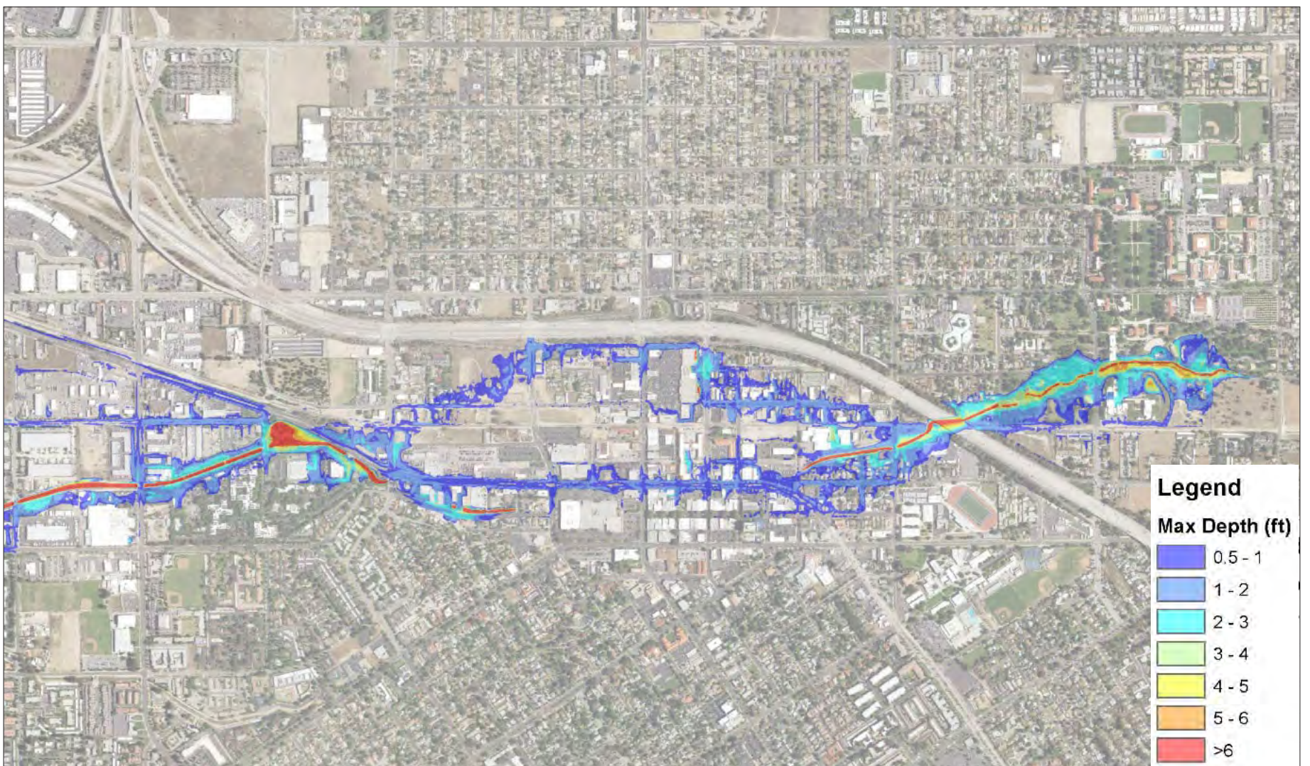
FIGURE 8-9. 100-YEAR FLOOD PLAIN WITH IMPLEMENTATION OF MPD ALTERNATIVE 1 (CULVERT IN REDLANDS BOULEVARD.)
