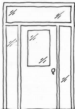
door with sidelights and transom
