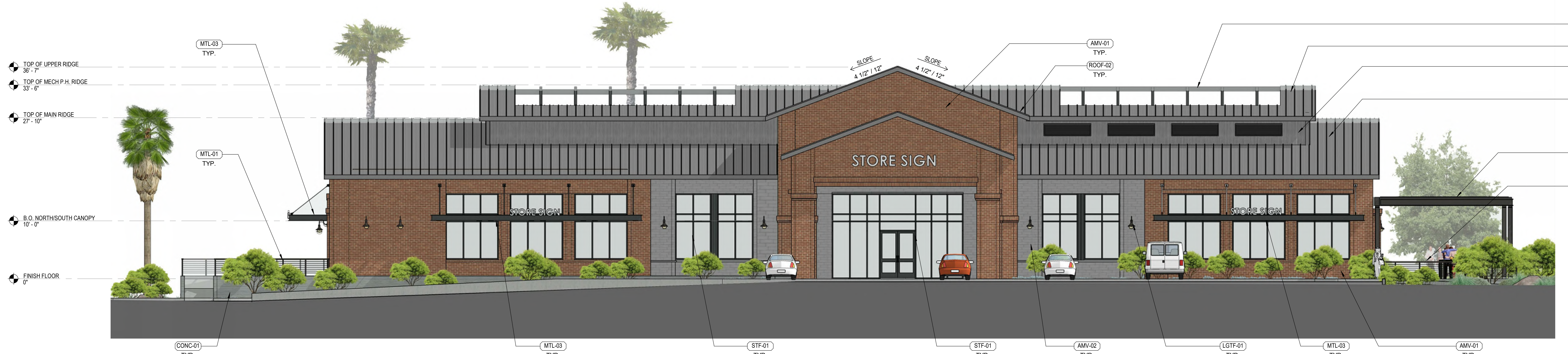
SOUTH ELEVATION - BUILDING A SCALE: 1/8" = 1'-0"
