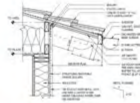
SAMPLE EAVE DETAIL AT ROOF TILE
