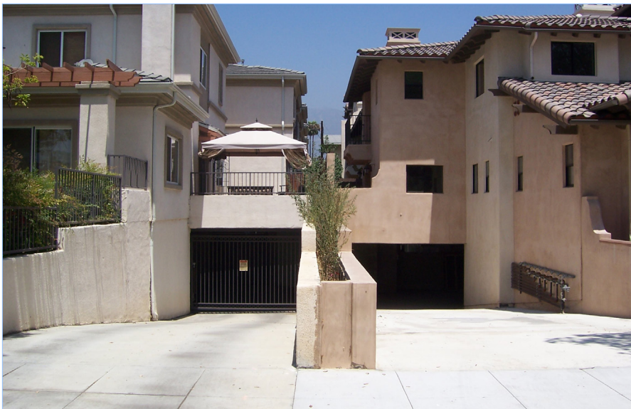
AVOID. The adjacency of these two multi-family residential parking entrances has a major impact on the pedestrian's perception of building. The mismatch in the size of the two respective openings compounds the problem.
