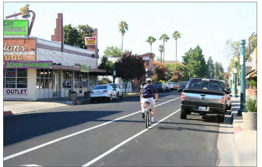
A Class II bike lane passes through a neighborhood-serving commercial district.
