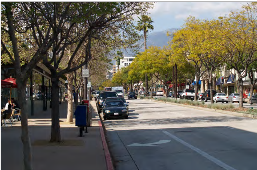
An arterial street with two lanes in each direction, a center median, and on-street parking
