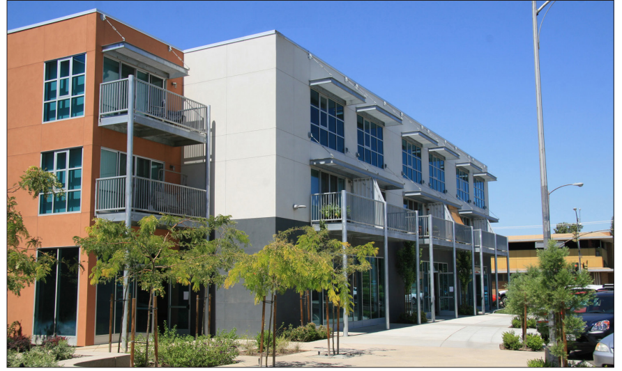
Volume on left side of building is set back from the rest of the building (horizontal articulation). Building is further articulated with protruding galleries and canopies (architectural projection) and paint color.
